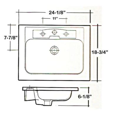
Dimensions of fixture are nominal and may vary within the range of tolerances established by ANSI Standard A112.19.2-2018. Dimensions and specifications subject to change without notice.
